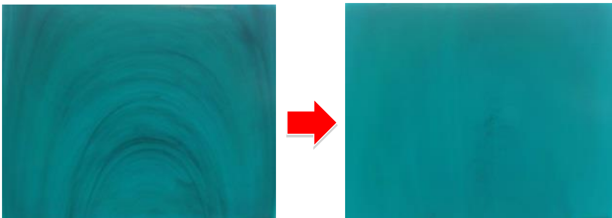
Figure 4: Flow lines in a plastic part can be avoided by using a mixing nozzle.
