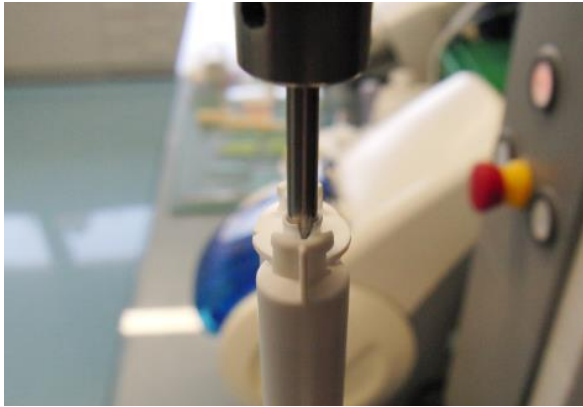
Figure 3: Weak area of a cartridge that could be eliminated with the use of a mixing nozzle
