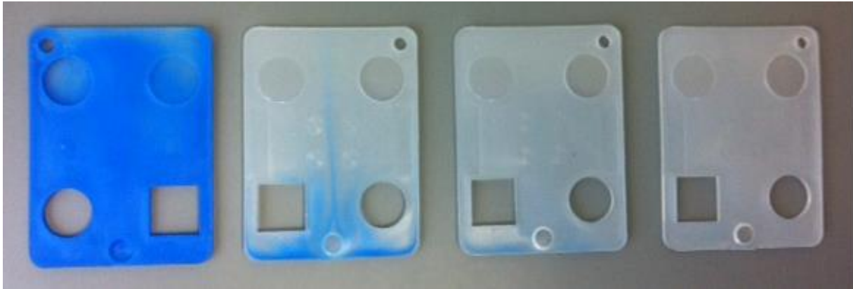
Figure 5: Promix mixing nozzles show effective inline self cleaning behaviour
