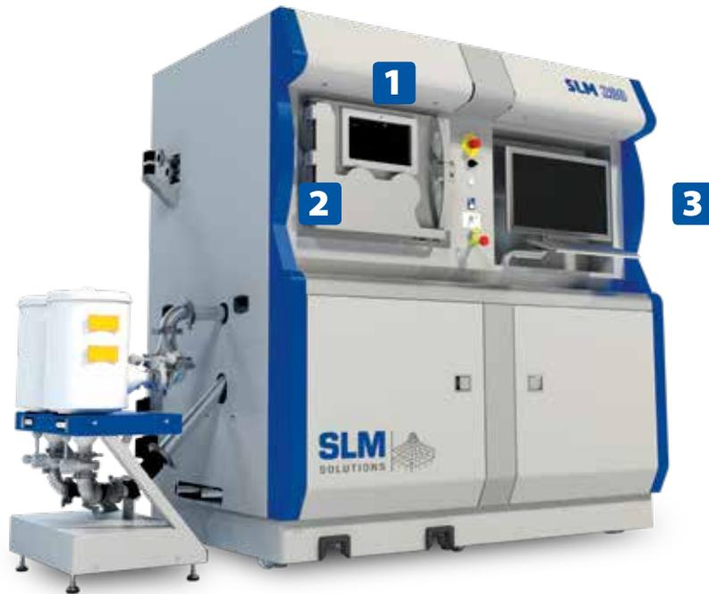
**1** Multi-laser technology was pioneered by SLM Solutions, who remain the market-leaders in multi-laser installations. The SLM<sup>®</sup>280 can be equipped with up to two 700W fiber lasers to accelerate the printing process of many metal additive powders.
