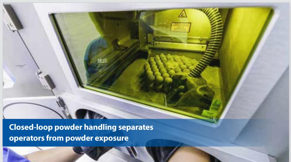
**Closed-loop powder handling separates operators from powder exposure**
